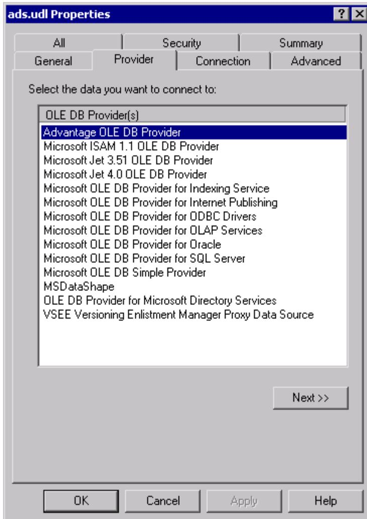
**Figure 22-3: Setting the connection string properties using a UDL file**
